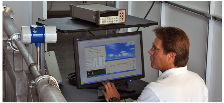
Calibration Technician performing an actual gas calibration in the flow laboratory.
