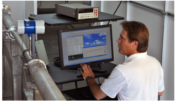
Calibration Technician performing an actual gas calibration in the flow laboratory.
