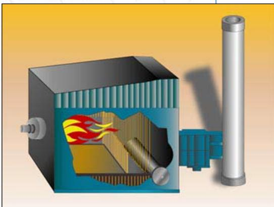
Sophisticated burner control systems optimize air/fuel ratio control to obtain peak thermal efficiency over the entire range of the burner, and to facilitate proactive emissions control. Mass flow control of air and fuel is used to automatically compensate for changes in temperature or pressure that affect combustion performance. Many systems also integrate fuel totalizing, air/fuel flow and valve position analog outputs for DCS interfacing, and remote system monitoring.
